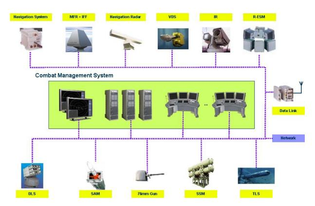
Figure 3 – Characteristic structure of a CMS
